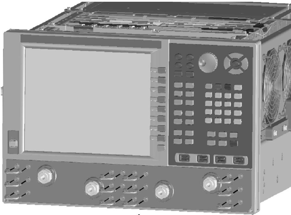
Figure 6 Front Panel Jumper Cables Installation
